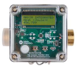
Accelerate your heat/flow meter development with our ultrasonic time-of-flight flow meter. MAXREFDES70 arrives with a complete ultrasonic flow measurement system, including piezoelectric transducers and spool body for both upstream and downstream pulsing. The system employs sophisticated DSP techniques to measure time-of-flight difference for a highly accurate flow rate calculation, especially at low flow rates.
